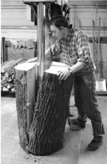
French coopers must split each timber by eye into stave-like widths, then trim each stave on a band saw closely following the grain, again by eye, with no guides or safety devices. American
