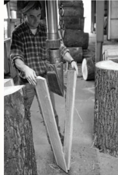
expensive. The staves are then stacked one layer for each barrel then left in the yard to season for two more years before returning to the cooperage for assembly and toasting.
